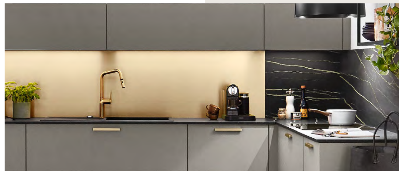
NVK 296 Yellow gold coloured This gold appearance is created on the basis of an HPL material with an integrated real metal foil. A stylish effect that combines wonderfully with gold-coloured accessories.
